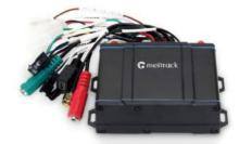
The MVT800 is a high end GPS tracker, that can handle multiple accessories at once. This type of model is ideal for larger vehicles such as freight and delivery vans. This particular model is one of the few that can be used to shut off the engine of the vehicle in case of theft.
