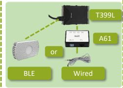
You can choose wireless or wired temperature sensor to monitor the temperature of the cold room in real time.
