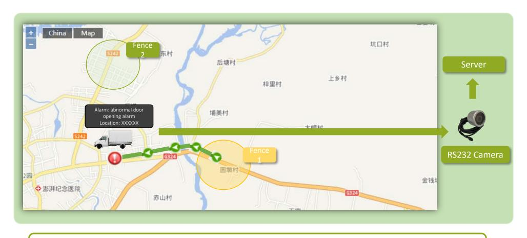
The driver is only allowed to open the door to unload in the designated area. The door sensor is used to detect the door opening status. If the door is detected to be opened outside the designated GEO-fence, an abnormal door opening alarm event will be uploaded. At the same time, the device will take pictures and upload them.
