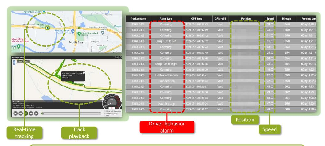
The driver's illegal driving behaviors such as speeding, rapid acceleration, rapid braking and sharp turns will be uploaded to the historical data report of the MS03 platform. The manager can confirm whether the driver's driving meets the safety standards based on these records.
