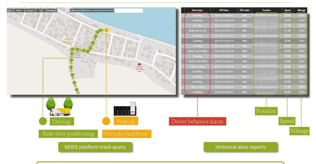
Users can view the real-time or historical track of the device on the Meitrack platform and use data reports to analyze the driver's driving behavior.
